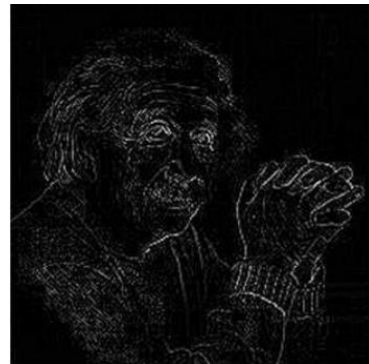
Image After applying Negative Laplacian operator
